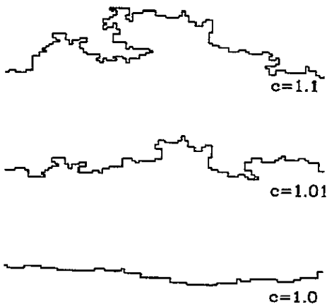
Figure 1. Domain walls in a two-dimensional random Ising ferromagnet ( L = 96 ) with the exchange couplings given by (1) for the three values of c indicated.
